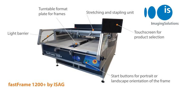
fastFrame 1200+ is a fully automated system for stretching small to extra large canvases. The machine is designed for the industrial mounting of large frames up to  $120 \times 120 \text{ cm}$  ( $48'' \times 48''$ ). It mounts up to 80 canvases per hour, depending on the size. This is several times faster than manual production.
