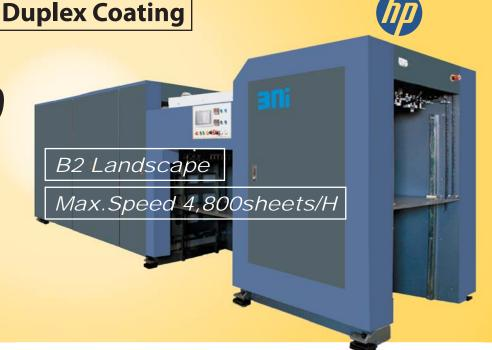
Digi Multi Coater/Duplex/H30 is Coater which is three in one system for Primer Coating as pre-processing before printing and UV/Water-based Varnish Coating after printing.
