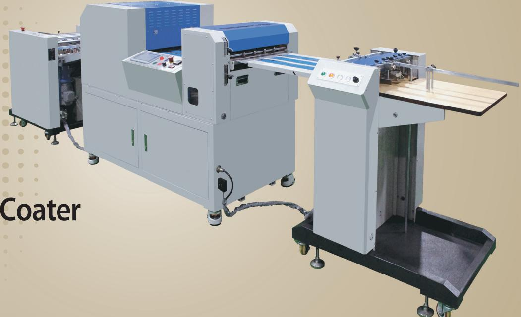
Digi Glass Coater is an UV coating machine that is totally new hologram transfer technology, which uses high precision glass cylinder system.
